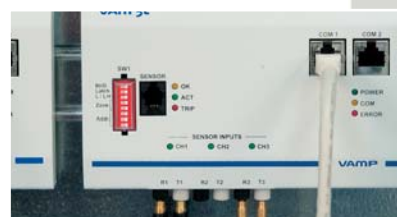
The arc sensor I/O units incorporate a snap-in connector for the portable sensor. The activated arc sensor channel is indicated with a led.
